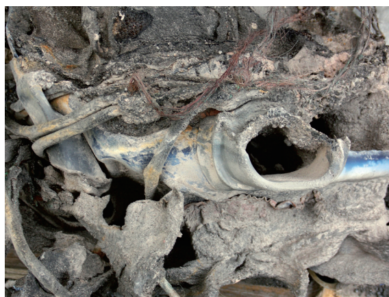
Figure 9. A sharp melting of polyethylene terephthalate used in common goods. The melting was less than 300°C.
