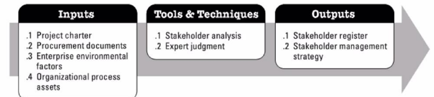
Figure 10-2. Identify Stakeholders: Inputs, Tools & Techniques, and Outputs
