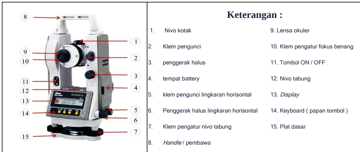
Gambar 2. 2 Bagian-bagian Theodolite
